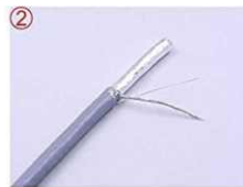
2 Sort shield braiding wires
