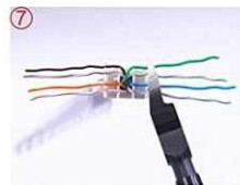
7 Cut off the needless cable edge
