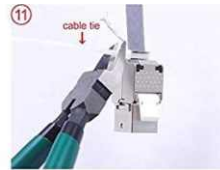
11 Push the cable line in and lock it, Cut off the excess braided and cable tie
