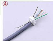
4 Put the cable through the pressure cover
