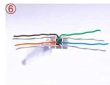
6 Aligning wire and press down. T568B is recommended
